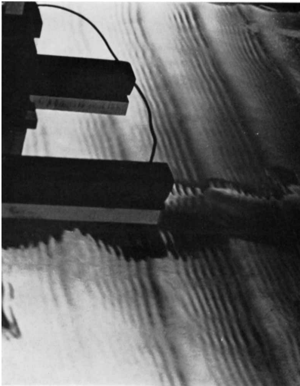
FIGURE 1. Fundamental wave with harmonic ripples. The wave maker frequency is 6.6 c/s. Note that the rippling is not confined to the front face, but appears all over the longer wave. Propagation is from right to left.
